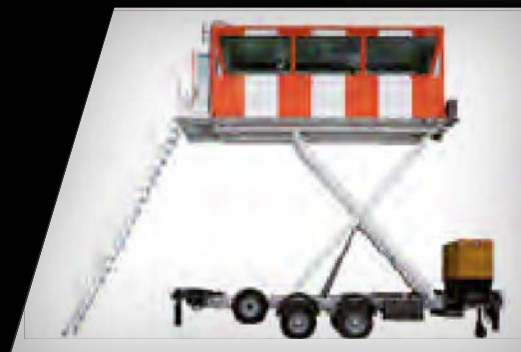
Mobile Air Traffic Control tower
