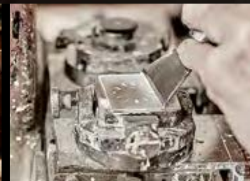
Printing the dialplate by tampon printing
